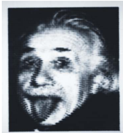
Figure 4. Reproduction of the famous photograph of Albert Einstein produced with the GSI raster scan system as a heavy ion beam TV using a 430 MeV/u carbon beam of 1.7 mm width (FWHM). The picture consists of 105 x 120 pixels filled by 1.5 \cdot 10^{10} particles given in 80 spills (5 sec. each) of the SIS accelerator. Original size of the picture: 15 cm x 18 cm. (Courtesy GSI.)
