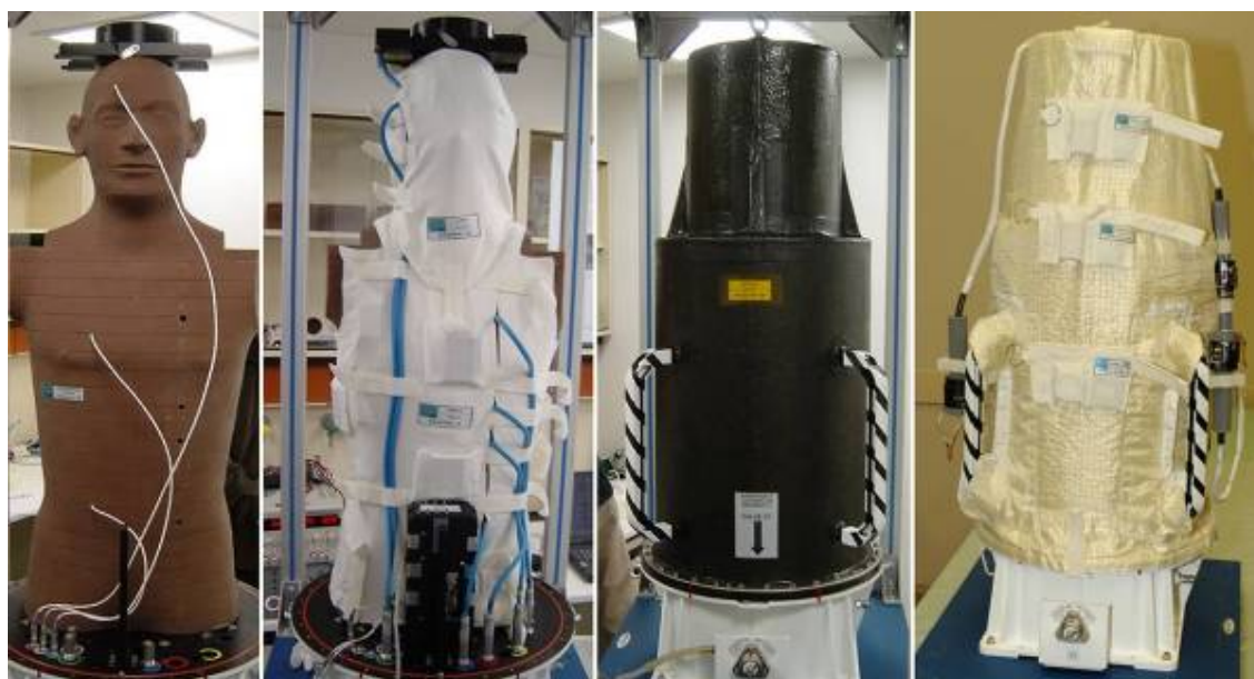
FIG. 2: The MATROSHKA phantom from left to right: A) anthropomorphic upper torso equipped with active detector systems, B) torso with poncho and hood equipped with passive detector systems for skin dose measurements, C) carbon fibre container to simulate the astronaut's space suit, D) facility ready for launch equipped with multi-layer insulation (MLI) for thermal protection
