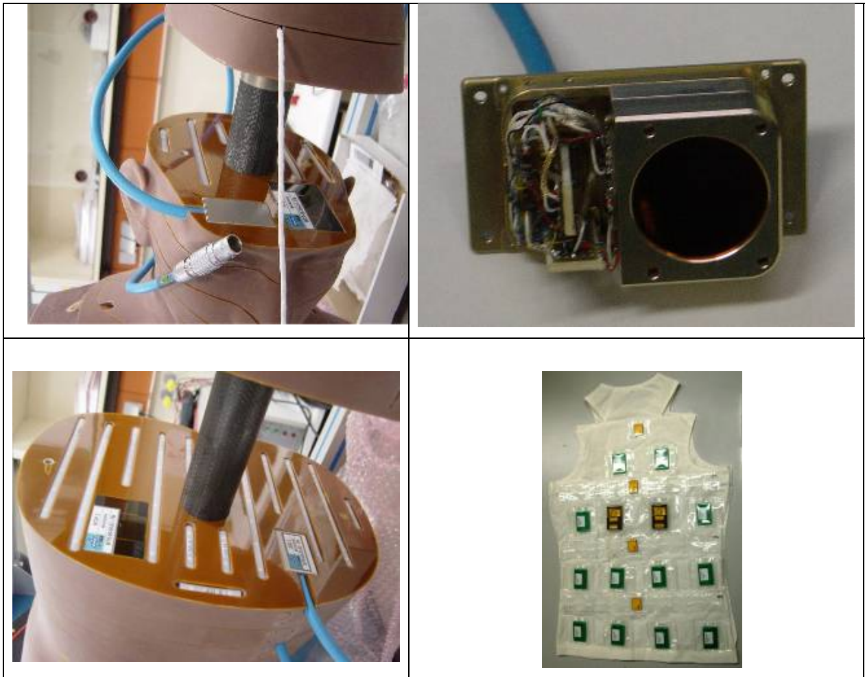
FIG. 3. A. View of the phantom head of MATROSHKA. It shows the head of the phantom with the integrated passive and active radiation detectors. Passive detectors are integrated in polyethylene tubes and in the “organ dose” packages. The sensor for the active Silicon-Scintillator Device (SSD) is shown with the blue cable connecting to the base structure. The white cable connects to a temperature sensor in the head of the phantom. B. DOSTEL sensor head which is mounted on the head of the phantom C. same as a, but section in the middle of the phantom was chosen. D. Phantom Poncho which is equipped with TLDs sewn in plastic stripes and neutron dosimeters. The pictures were taken during detector integration prior to the launch of the facility.
