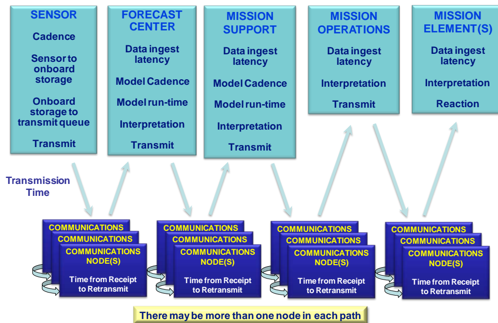
Figure 11: Illustration of components of an end-to-end communications infrastructure, with an indication of factors that contribute to the timeliness of actionable response.
