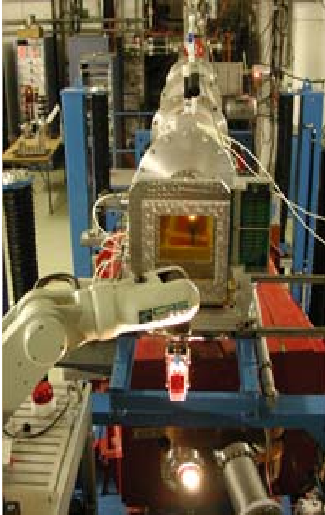
The high-energy irradiation facility in Cave A. The robotic arm moves the samples (in flaks) to the beam position for the required exposure time. Beam is delivery by spot-scanning of the flask. This is a generally-purpose facility for irradiation of in vitro samples with high energy heavy ions.
